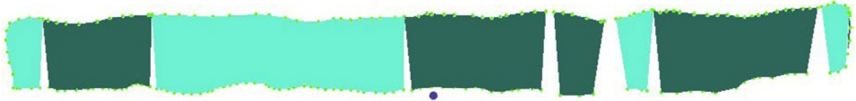
FIGURE 20 – (SCREEN-CAPTURE OF A 3D DRAWING; SECTION PERSPECTIVE) THIS IMAGE WAS CAPTURED AFTER THE DRAWING PROCESS HAD BEEN COMPLETED. A MAJOR DRAWBACK OF DRAWING IN 3D WITH POLYGONS IS THAT THE POLYGON IS PROJECTED AS INDIVIDUALLY SEGREGATED PIECES—NOTE THE SHADING DIFFERENCES AND MOST SIGNIFICANTLY THE SEVEN WHITE SPACES BETWEEN. (IMAGE BY J.J.L. KIMBALL 2014; 3D DRAWING BY J.J.L. KIMBALL 2014).
