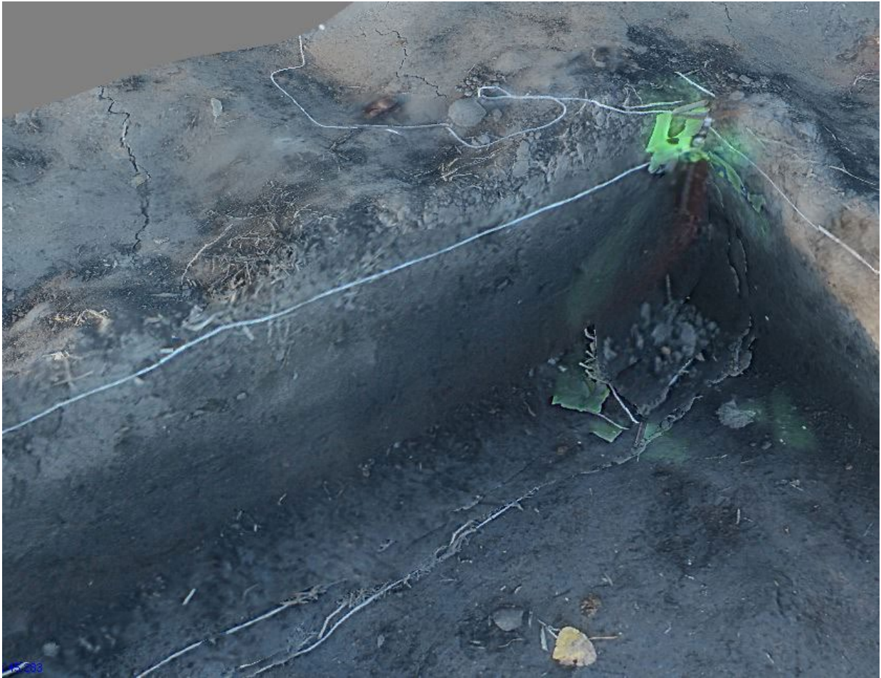
FIGURE 34 – (SCREEN-CAPTURE OF A 3D MODEL) THE CONSEQUENCE OF NOT PREPARING THE SITE BY REMOVAL OF ITEMS NON-ESSENTIAL FOR THE PHOTOGRAPHIC PROCESS. VISIBLE ARE MULTIPLE PROJECTIONS OF ONE STRING, A NEON STRIP OF TAPE, AND A HINT OF RED IN THE CORNER OF THE TRENCH FROM A RANGE POLE. (IMAGE BY J.J.L. KIMBALL 2014; 3D MODEL BY J.J.L. KIMBALL 2014).
