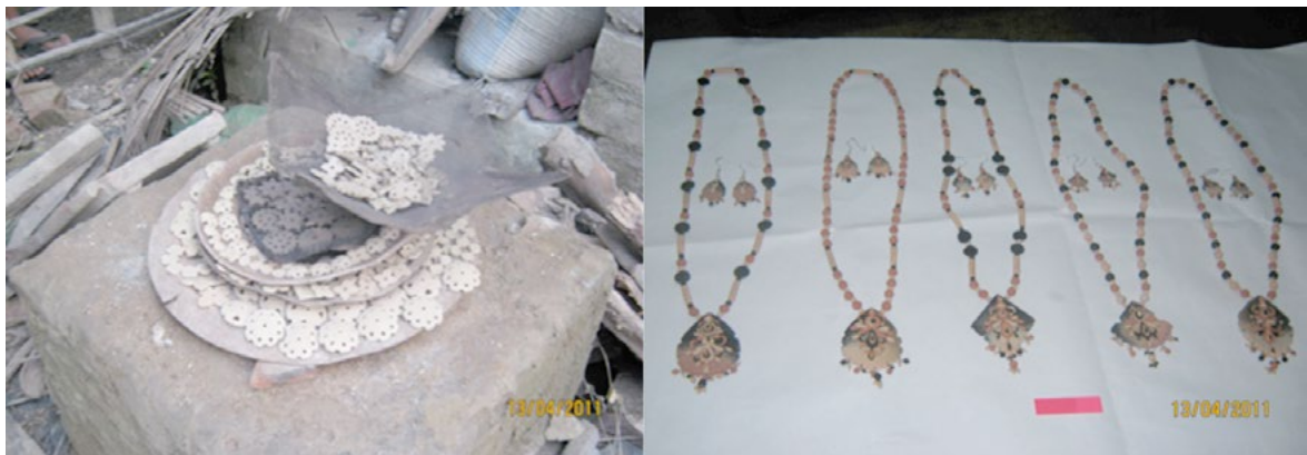
FIGURE 3. THE FIRING PROCESS OF THE ORNAMENTS, AND THE FINAL RESULTS
